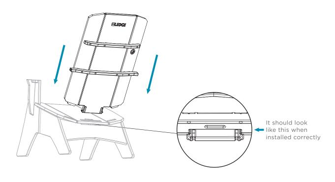
**STEP 7:** Attach the armrest by inserting the front 2 screws.
