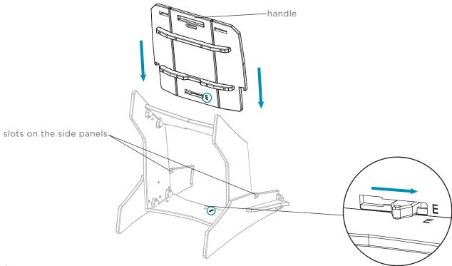
**STEP 6:** Slot the back rest into place.
