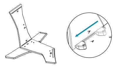
**STEP 3:** Insert side B of the back panel into slot B on the right side panel. Then slide two keys into place and secure with a screw.
