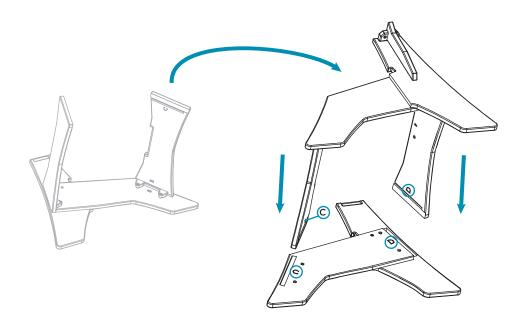
**STEP 5:** Lay the assembly on the ground with the back panel showing the letter E facing up. Grab the seat by the handle and lower it onto the slots on the side panels. Then, insert a key into slot E located on the underside of the seat, slide the key to the right, and screw it in place.
