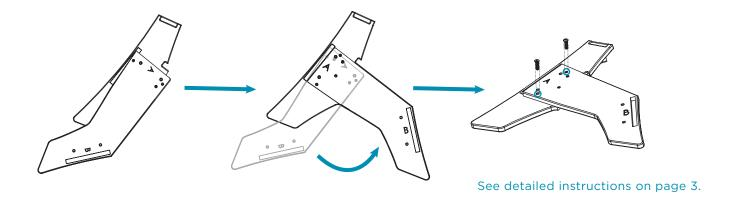
**STEP 2:** Insert side A of the front panel into slot A on the right side panel. Then slide two keys into place and secure with a screw. There will be some flex until the base is fully assembled.
