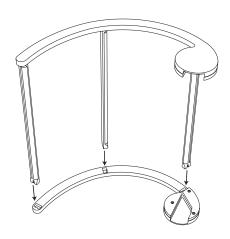
**STEP 4:** Slip fabric on to the frame with the clear media viewing window facing the inside of the curve, or the bottom of the shade. Close velcro flap.
