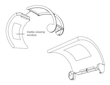
**STEP 5:** Slide frame on to the back of seat. In some cases there's a gap between the seat and shade, this is normal as long as shade feels secure.
