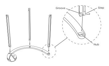
**STEP 3:** Set the second frame piece on top, repeating the process of inserting the tabs into the holes, and apply pressure to lock them together.
