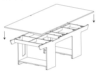
**STEP 8:** Locate the (20) keys you have already inserted into the table and screw them into place using the included Allen screws and Allen wrench.
