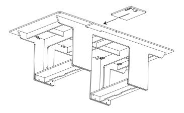
**STEP 10:** Secure the drawers with the T-shaped keys and screws.
