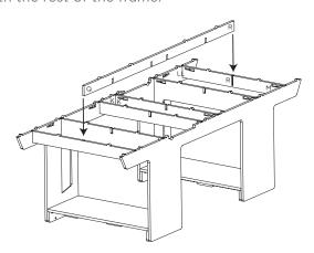
**STEP 6:** Insert the (20) keys into the key slots located on the brackets. Do not screw the keys into place until step 8.
