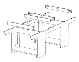
**STEP 5:** Align the corresponding letters of the long crossbar and insert the piece into the table frame. Slide the pieces together, using a mallet if needed. Continue until the top of the long crossbar is flush with the rest of the frame.
