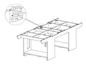
**STEP 7:** Place the table top on top of the frame. Adjust slightly until the grooves on the bottom of the table align and the table rests properly on the table frame.
