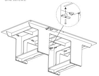
**STEP 11:** Slide the side of the net with a hook tab into the notch of the table top. Push down on the other side to lock into place.
