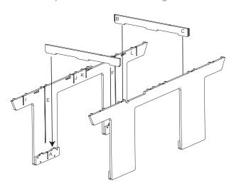
**STEP 2:** Align the corresponding letters of the shelves and drop them on the L-slot tabs. Slide inward until it locks into place, using a mallet if needed.
