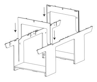
**STEP 4:** Align the corresponding letters of the top crossbars and insert them into the table legs. Slide the pieces together, using a mallet if needed. Continue until you have inserted all four crossbars (two middle crossbars, two end crossbars) into the table legs and the tops are flush.
