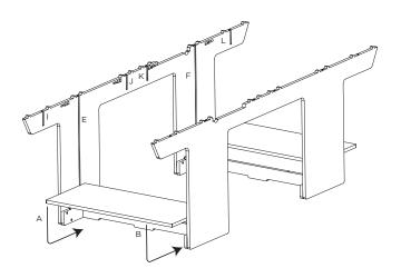
**STEP 3:** Align the corresponding letters of the two brackets and insert them into the table legs. Slide the pieces together, using a mallet if needed.
