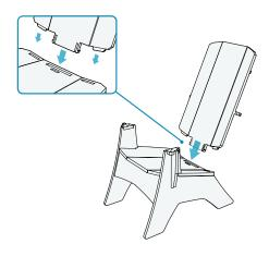
**STEP 2:** Starting with either side, position the armrest onto the base, aligning with the front screw hole. Using the hex screwdriver, assemble using (1) screw in the hole.
