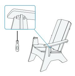
**STEP 3:** Align the rear screw holes. Assemble using (1) screw.
